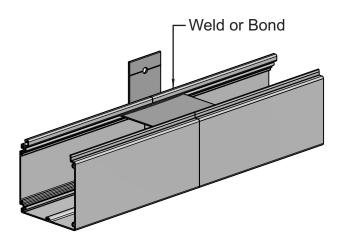
**4.)** Weld or bond both sides of the top and bottom brace/bracket to secure the splice.
