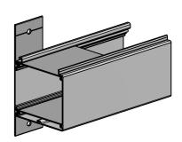
**2.)** Insert brace/brackets into the top and bottom of one section of raceway. Brace/brackets should be flush with the edge of the raceway.
